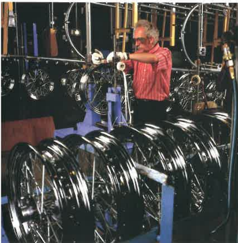
▼ FIGURE 11-8 BULK-GAINING: FABRICATED METAL PRODUCTION Motorcycle wheels are fabricated at the Harley-Davidson factory in York, Pennsylvania.
