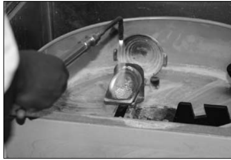
A Jewelry I student (above) heats molten bronze using an oxy propane torch.
